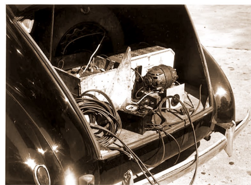
Like father, like son - Alan's father John's Ford sedan with a "studio in a trunk": A 1933 state-of-the-art, 315 pound (143 kg) aluminum disk recorder that was used to record Huddie Ledbetter , better known as " Lead Belly ".
